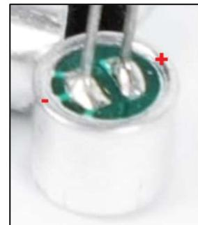
You can also use a digital multimeter in continuity mode to find which leg is electrically connected to the shell. This will also be the negative pin.
