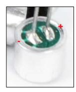
You can also use a digital multimeter in continuity mode to find which leg is electrically connected to the shell. This will also be the negative pin.
